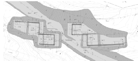
MSEW foundation area excavation layout
