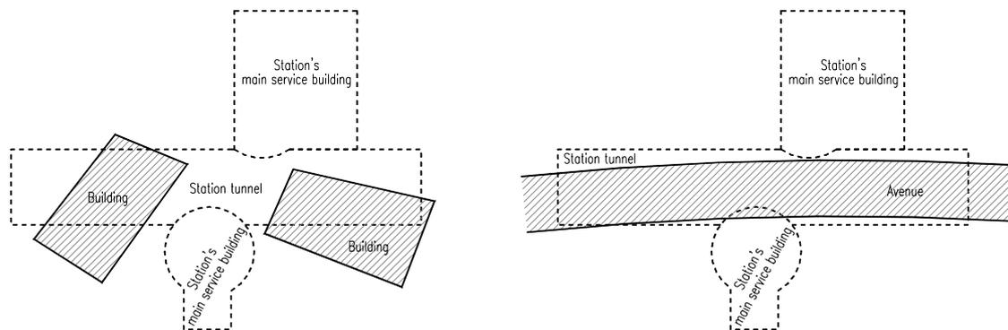
Figure 1. Layout of a typical underground station – Case A, buildings along tunnel's axis – Case B, significant avenue along tunnel's axis
