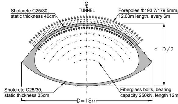
Figure 2. Geometry of tunnel and temporary support measures – Top Heading
