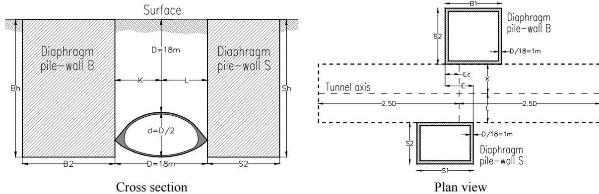
Figure 3. General geometrical layout for analysis
