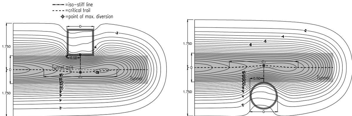
Figure 9. Tunnel-induced surface settlements– Critical trail and iso-stiff line – Sp1model3 and Sp1model4
