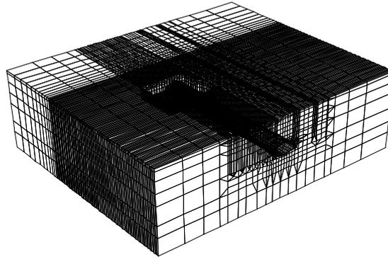
Figure 5. Typical part of a 3D finite-difference grid
