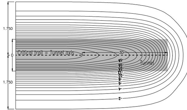
Figure 8. Tunnel-induced surface settlements – Critical trail – Sp1model2
