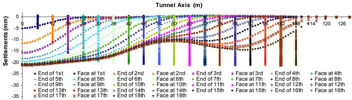
Figure 12. Development of longitudinal surface settlement profile with tunnel progress for analysis sp1modell
