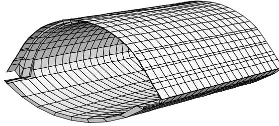
Figure 6. Typical view of the simulated 3D tunnel's shotcrete shell
