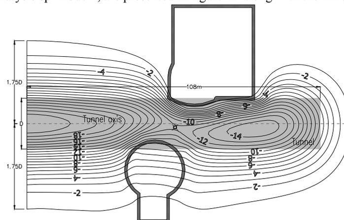
Figure 11. Tunnel-induced surface settlements – Point of inflection – Sp1model1
