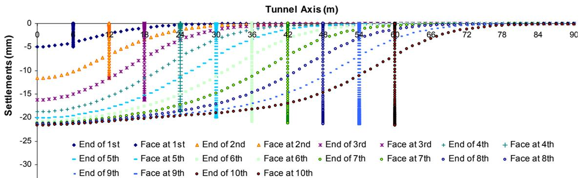
Figure 7. Development of longitudinal surface settlement profile with tunnel progress for greenfield analysis sp1model2
