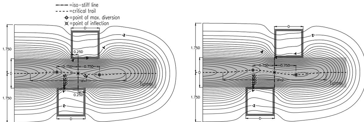
Figure 10. Tunnel-induced surface settlements – Critical trail and iso-stiff line – Sp1model5 and Sp1model6
