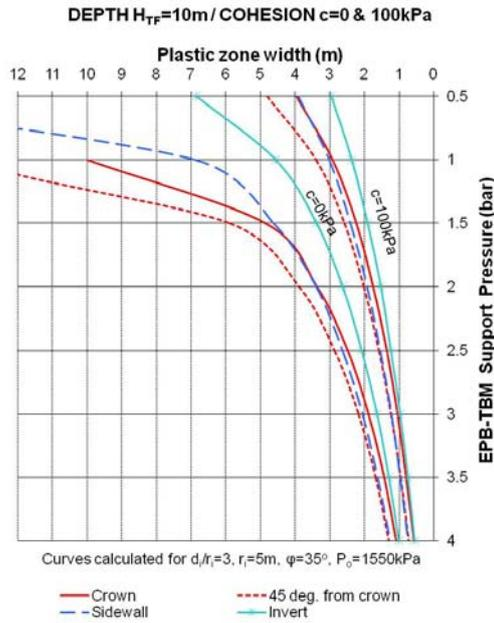
Figure 7. Plastic zone width for  $P_o=1550$  kPa,  $c=0$  & 100 kPa &  $H_{TF}=10$  m
