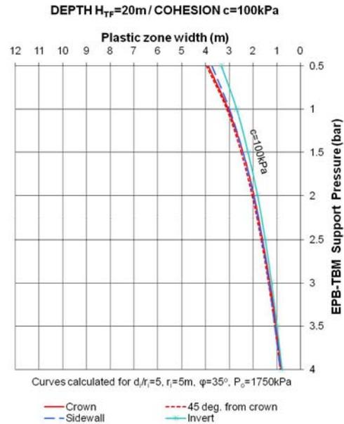
Figure 8. Plastic zone width for  $P_o=1750$  kPa,  $c=100$  kPa &  $H_{TF}=20$  m
