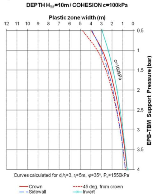
Figure 6. Plastic zone width for  $P_o=1550$  kPa,  $c=100$  kPa &  $H_{TF}=10$  m
