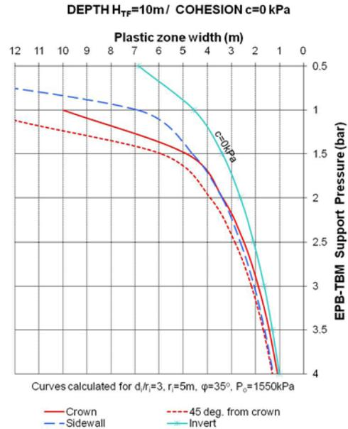
Figure 5. Plastic zone width for  $P_o=1550$  kPa,  $c=0$  kPa &  $H_{TF}=10$  m
