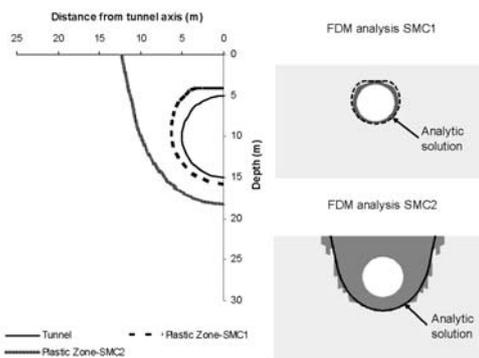
Figure 3. Analytic solution and FDM analysis results: closed-form solution validation (Massinas et al, 2009)
