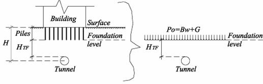
Figure 4. Physical and equivalent model for analytical calculations
